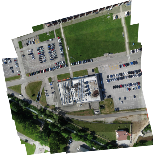
FIGURE 7.10: Dataset 2: Mosaic obtained after image alignment, with no colour correction and seamline optimization.
