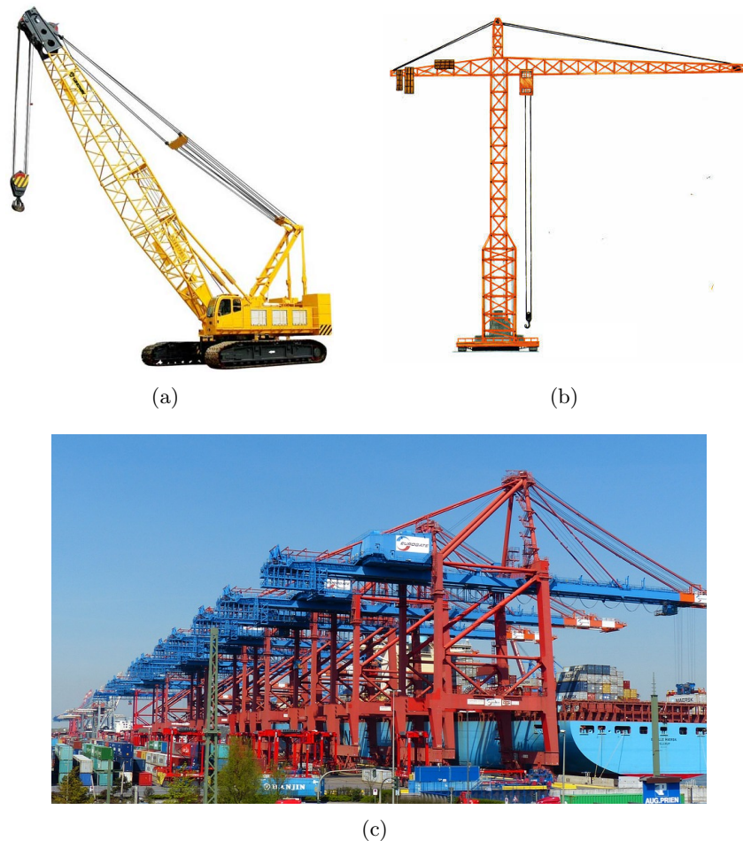
Figure 5.1: Crane devices: mobile crane (a), tower crane (b) and gantry cranes (c).
