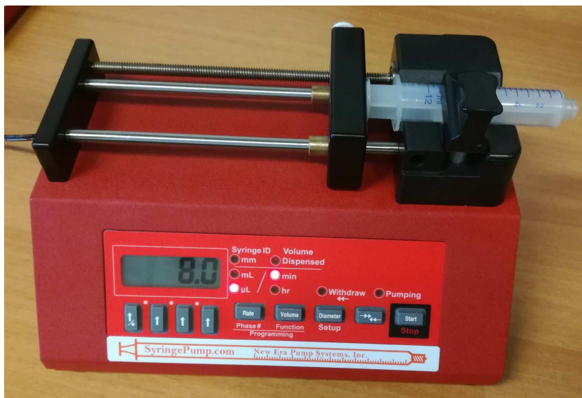
Figure 2.16: Photo of the NE-300 automated syringe pump used for injecting the fluids in the experiments.
