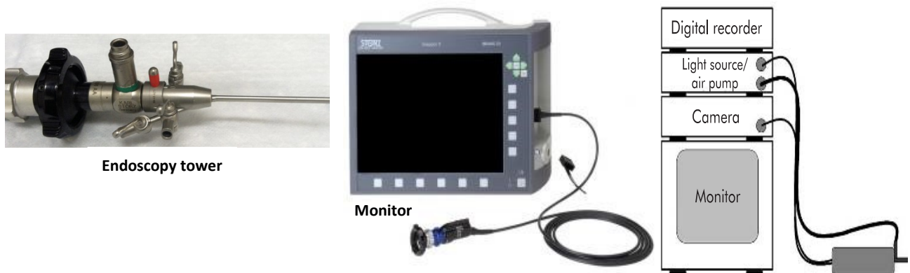
Figure 39: Specific instrumentation use to perform endoscopy. This coloview endoscopy system endoscopy allows to perform a video-controlled direct analysis into the colon of living mice; the endoscopic tower is fiber optic light transmission incorporated and provides a bright and magnified view of the colon mucosa into the monitor.
