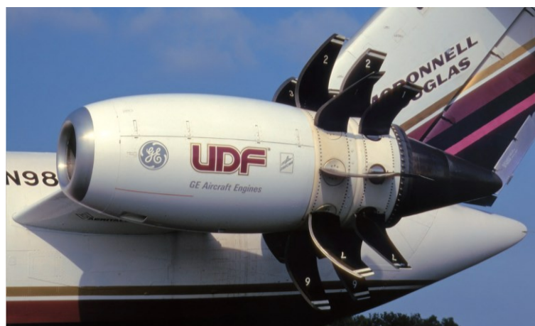
Figure 1.1 – Contra-rotating Open Rotor in pusher configuration. General Electric UDF® (UnDucted Fan) mounted on a McDonnell-Douglas MD-80.
