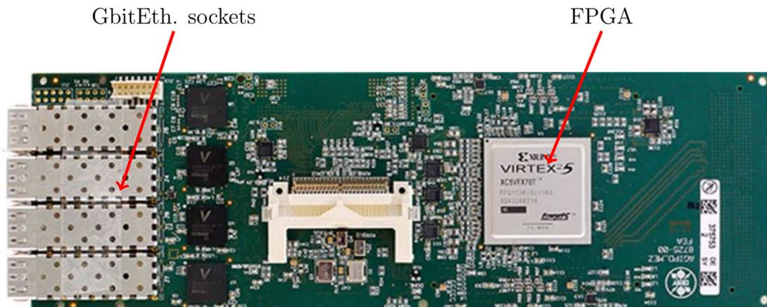
Figure 3.10: The mezzanine board with a Virtex-5 XILINX FPGA and four GBit Ethernet sockets for the data connection.
