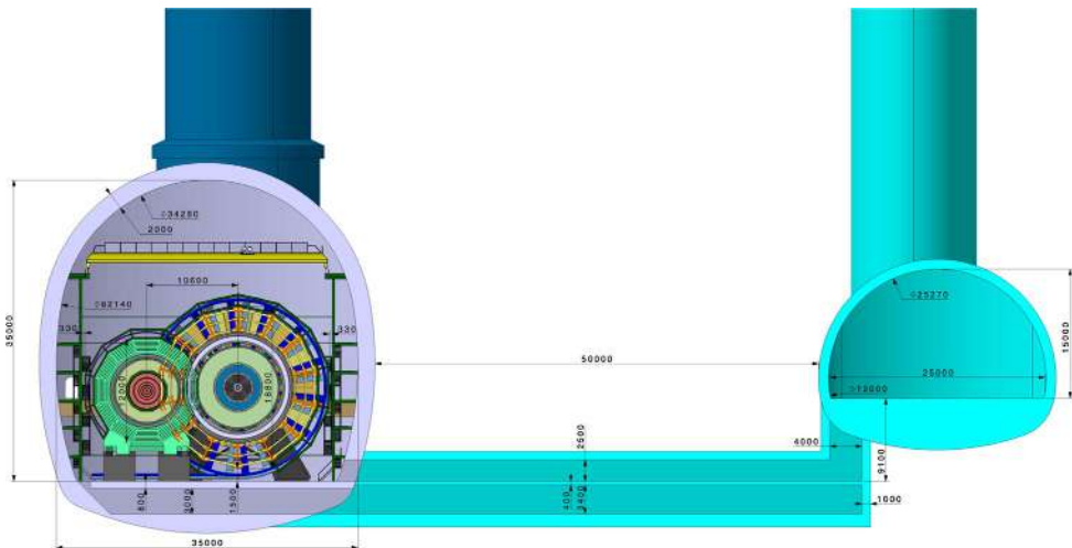
Fig. 7.5. Sketch of FCC-ee detector CLD inside the experiment cavern (left side of cavern, in green, yellow and red), along with a subsequent, larger FCC-hh detector (right side of cavern, in blue, yellow and orange).
