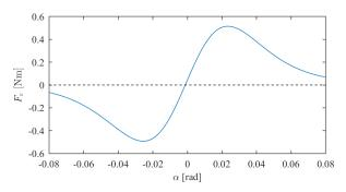
**Figure 7.** Behavior of  $F_{\varepsilon f}$  in relation to master/slave misalignment angle  $\alpha$ .
