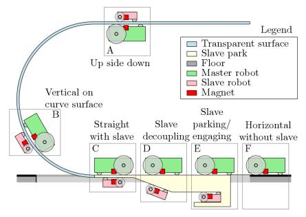
Figure 2. System description and illustration of different operation phases.
