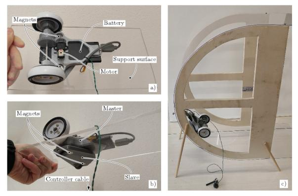
**Figure 15.** Functional prototype with nonmagnetic transparent support sheet. (a) Top view highlighting position of the master and its main component; (b) bottom view portraying the slave. The controller (a switch-potentiometer setup) is off-screen. (c) Experiment 2 setup, with robot located at approximately  $\vartheta = -\pi/4$ .
