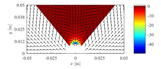
**Figure 3.** Morphology of  $\mathbf{F}_m$  field. In the chart, magnetic moments  $\mathbf{m}_r$  and  $\mathbf{m}_f$  are vertically aligned. Moment  $\mathbf{m}_r$  is placed at coordinates (0,0). Direction of force acting on the second dipole, shown with arrow plot; magnitude of vertical component of the same force, shown in color-coded chart. White area, upward vertical components (i.e., repulsive).
