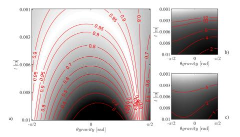
**Figure 11.** Traction margin  $T_{\mu}$  and contact forces on a curved surface against thickness t and angular position  $\vartheta_{gravity}$  along the curved path. (a) Traction margin; contact force for (b) the wheels in  $\mathbf{P}_{0,r}$  and (c) the skid in  $\mathbf{P}_{1,r}$ .
