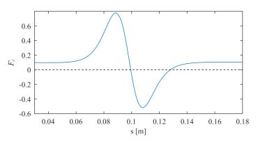
**Figure 5.** Behavior of  $F_{\varepsilon f}$  in relation to master/slave misalignment distance s.
