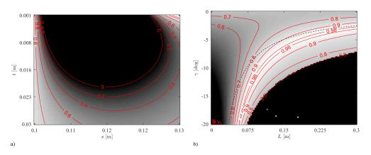
**Figure 14.** Traction margin during parking; (a)  $T_{\mu}$  during proper parking phase (Phase E) against misalignment *s* and thickness *t*; (b)  $T_{\mu}$  during ramp overcoming (Phase D) against travel *L* and ramp angle  $\gamma$ ; dashed line:  $L = L(t_{park} = 0.020)$ , i.e., the value that *L* should have to reach  $t_{park} = 0.020$  mm.
