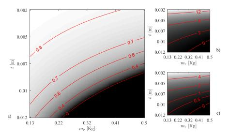
**Figure 13.** Traction margin  $T_{\mu}$  and contact forces during ceiling operation in upside-down condition against mass  $m_r$  of the robot and thickness *t* of the support sheet. (**a**) Traction margin; contact force for (**b**) wheels in **P**<sub>0,r</sub> and (**c**) the skid in **P**<sub>1,r</sub>.
