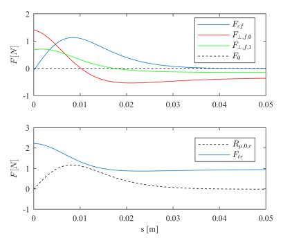
**Figure 9.** Development of forces as a function of *s* during the parking or coupling phase. Dashed line: inferior limit for the curves.
