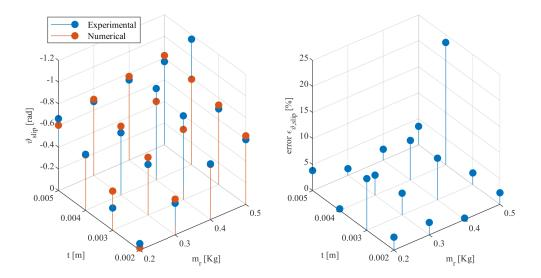
**Figure 17.** Comparison between numerical results of the model and results from Experiment 2. **Left** plot: data points for different robot masses  $m_r$  and for different thicknesses t for both the numerical and experimental campaigns; note that the z-axis is flipped. **Right** plot: relative error between numerical and experimental values, normalized with respect to  $\pi/2$ .
