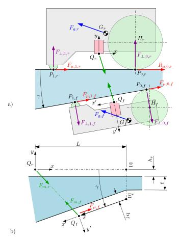
**Figure 4.** Straight-surface master–slave interaction. (a) Physical implementation of the actors; (b) geometrical relation between forces and parameter *s*. Note that friction forces  $\mathbf{F}_{\mu,0,f}$  and  $\mathbf{F}_{\mu,1,f}$  are represented by a single vector  $\mathbf{F}_{\mu,f}$  for simplicity.
