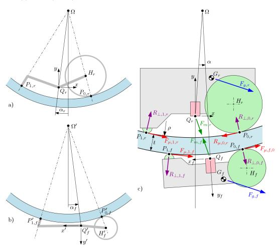
Figure 6. Master robot and slave on a cylindrical support sheet. (a) Master with respect to axis Ω; (b) slave in its local frame of reference; (c) whole system in the frame of reference of the master robot.
