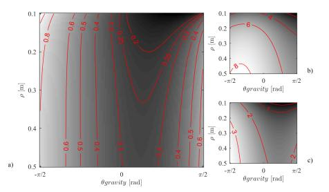
**Figure 12.** Traction margin  $T_{\mu}$  and contact forces on a curved surface against curvature radius  $\rho$  and angular position  $\vartheta_{gravity}$  along the curved path; (**a**) traction margin; contact force for (**b**) the wheels in **P**<sub>0,r</sub> and (**c**) the skid in **P**<sub>1,r</sub>.
