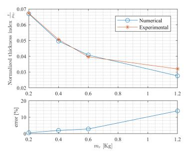
**Figure 16.** Comparison between numerical and experiment results (Experiment 1). Top plot: data points for different robot masses  $m_r$ ; below plot: relative error.
