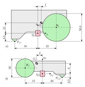
Figure 10. Geometry and dimensions of the robots. (a) Master and (b) slave.
