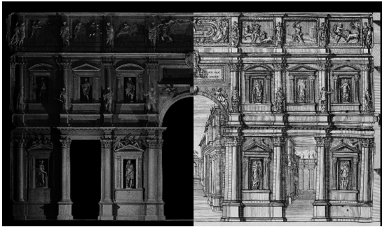
Fig. 5. Comparison between the laser scanner pointcloud (left) and the measured drawing by Bertotti Scamozzi and presented in his book Le fabbriche e i disegni di Andrea Palladio , Vicenza 1776
