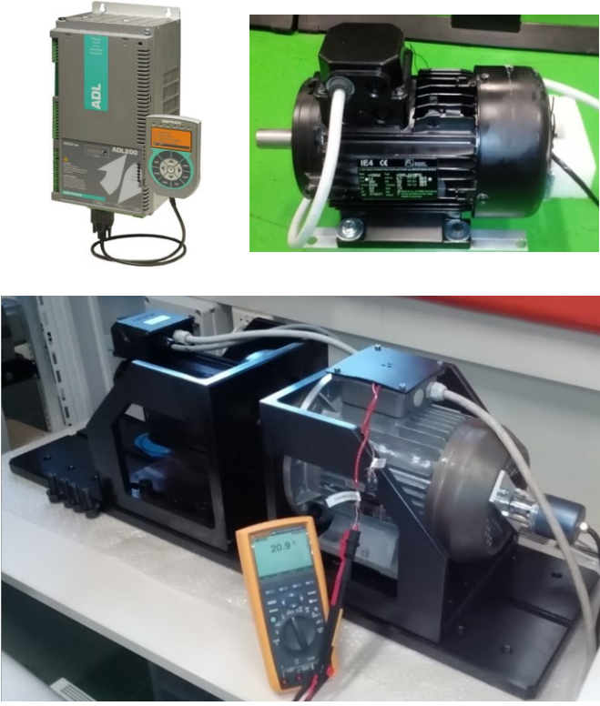
Fig. 3. SynRMs adopted in the experimental tests: industrial drive and motor #1 (top), motor #2 and test-rig (bottom).
