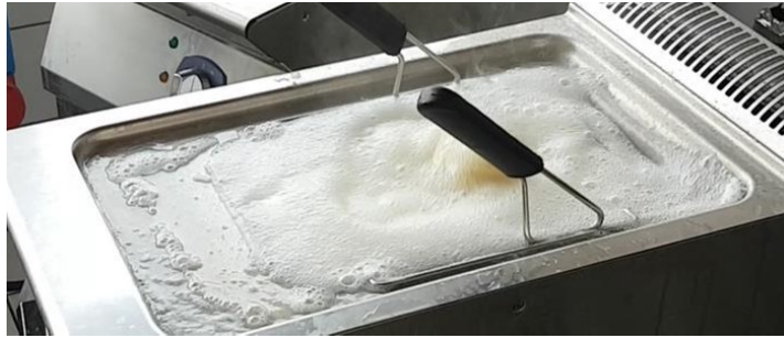
Figure 5.4. Foam formation during cooking at the 7 batch of continuous cooking.
