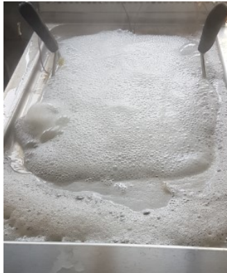
Figure 6.9. Picture of foam layer causing the water to go into the overflow drain at power rating of 6 kW.
