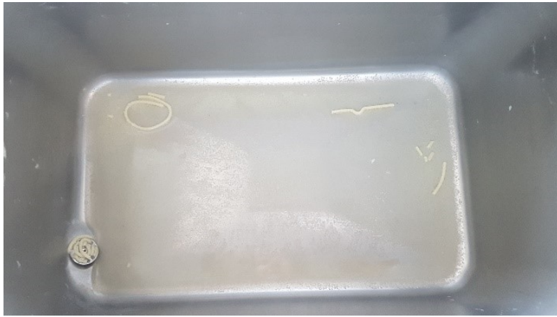
Figure 5.8. Adhering starchy layer to the well surface of the pasta cooker after continuous cooking of 12 batches.
