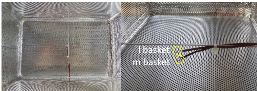
Figure 6.5. Internal side of basket with the wire supporting the l- and m- basket probes.
