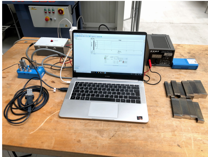
Figure 3.15: 3 rd DoE's specimens static compliance assessment – data acquisition
