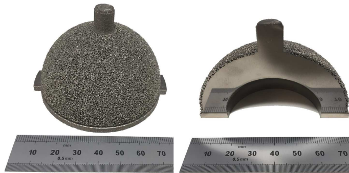
Figure 1.28: AM acetabular hip prosthesis: lattice structure enhances bone ingrowth [60]
