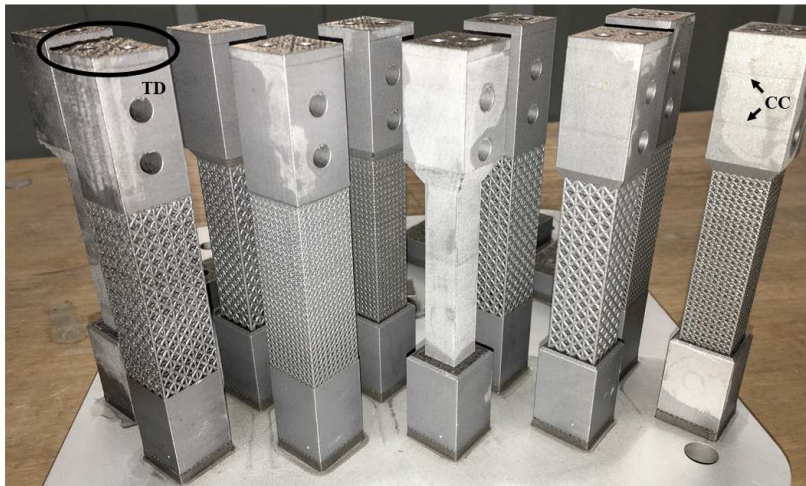
Figure 2.7: Macroscopic defects of AlSi10Mg specimens (TD: thermal deformation, CC: inert gas filter cleaning cycle)
