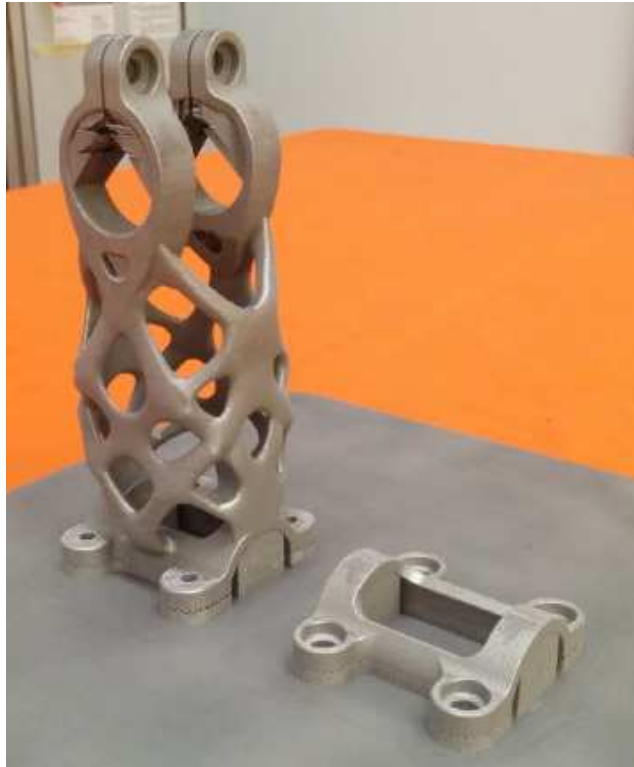
Figure 1.46: SLM-manufactured titanium alloy optimized bike stem (LAMA FVG™)
