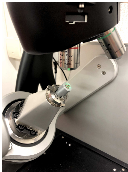
Figure 3.9: FBCCZ lattices geometric accuracy assessment – section measurement
