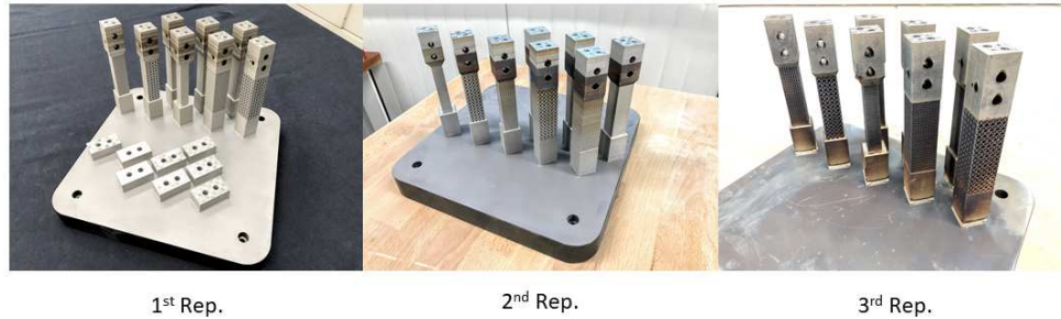
Figure 2.15: As-built SLM-manufactured SS 316L specimens and masses
