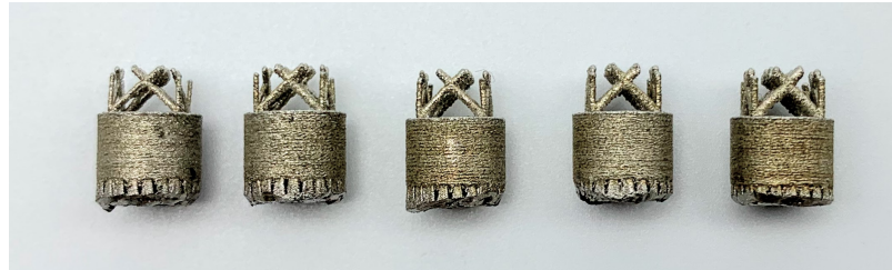
Figure 3.8: FBCCZ lattices geometric accuracy assessment – effective beam section
