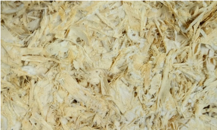
Figure 6.1: Compostable insulation material MycoFoam®. The material is composed by wooden scraps, bounded by mycelium (fungi's roots).
