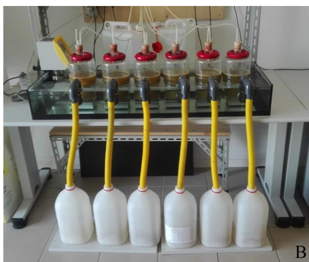
Figure 7. Rumen simulation technique (Rusitec, A) and the fermenter developed at the University of Udine (Mason et al., 2015, B)
