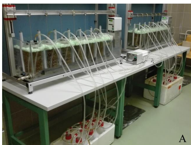
Figure 7. Rumen simulation technique (Rusitec, A) and the fermenter developed at the University of Udine (Mason et al., 2015, B)
