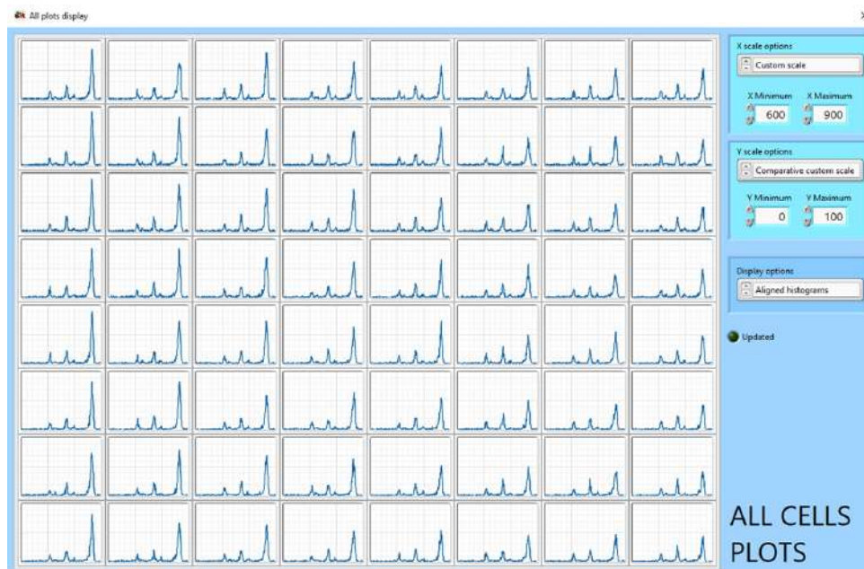
FIGURE 4.22: FICUS software screenshot of the simultaneous live acquisition of the 64 channels of the Detector System of the signal coming from the calibration sample: all channels work properly.
