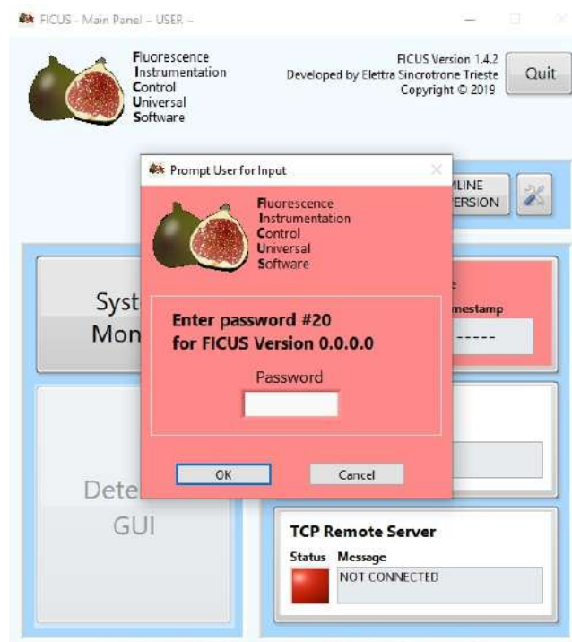
Figure 32: The FICUS control window: to pass from the FICUS software User version to the Beamline Staff version.
