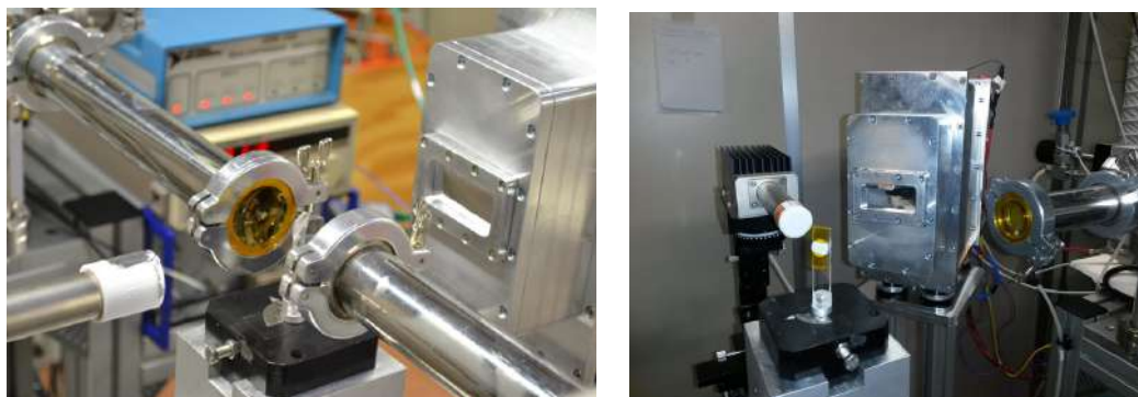
FIGURE 4.16: The detector system during the test at the XAFS beamline: (a) our detector system and the KETEK SDD are both in normal position. (b) the KETEK sensor is in normal position while our detector system is in parasitic position.
