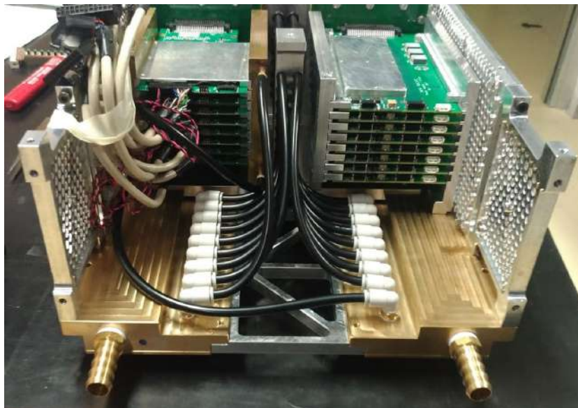
FIGURE 4.8: Detail photo of the cooling system of the detector system (system being assembled). It is possible to see: inlet and outlet cooling distribution, BE heat exchangers, and the tubes through which the refrigerated fluid flows.
