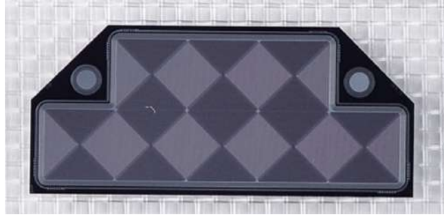
FIGURE 5.2: The multipixel SDD with trapezoidal shape for the detector system TwinMic. The active area of each sensor is divided into 8 square elements; the long base of the detector measures 33.6 mm, the short base 20.3 mm and the height 15 mm [30].
