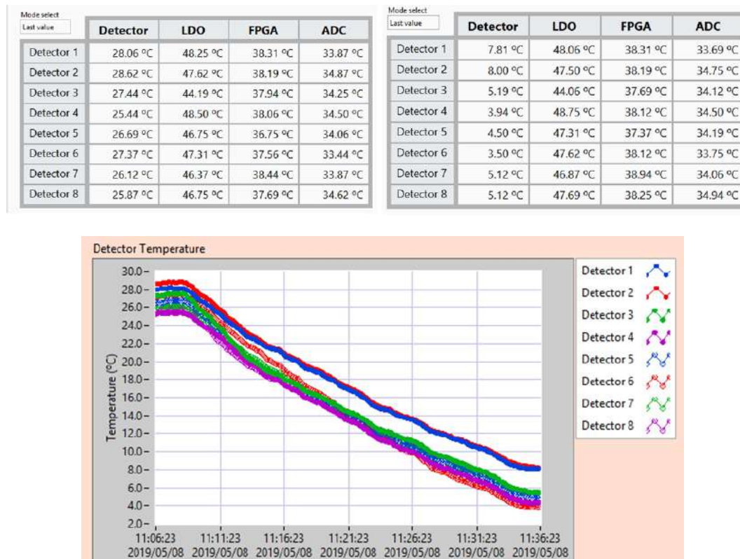
FIGURE 4.23: (a) Typical values of the temperatures in the condition at room temperature ( T_{amb} ) and in the condition of cooled system ( T_{cool} ) (b) The progressive trend of the temperatures during the gradual feeding phase of the Peltier cells.
