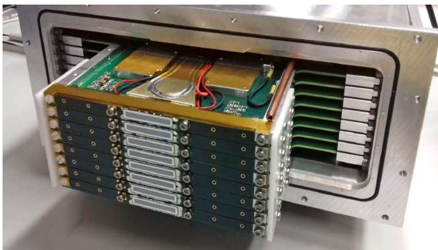
FIGURE 4.20: The SDDs installed in the XAFS-SESAME Detector System.
