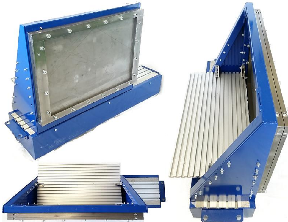
Figure 5.1. Test setup with a rectangular plate for the implementation of the velocity feedback loop system with inertial actuators.
