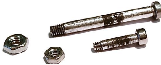
Figure 3.26. Screws used as shafts in the hinged prototype with visible wear effect.
