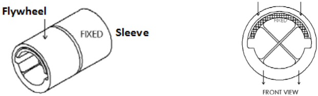
Figure 3.11. Position of the flexural bearings in the flywheel and sleeve.
