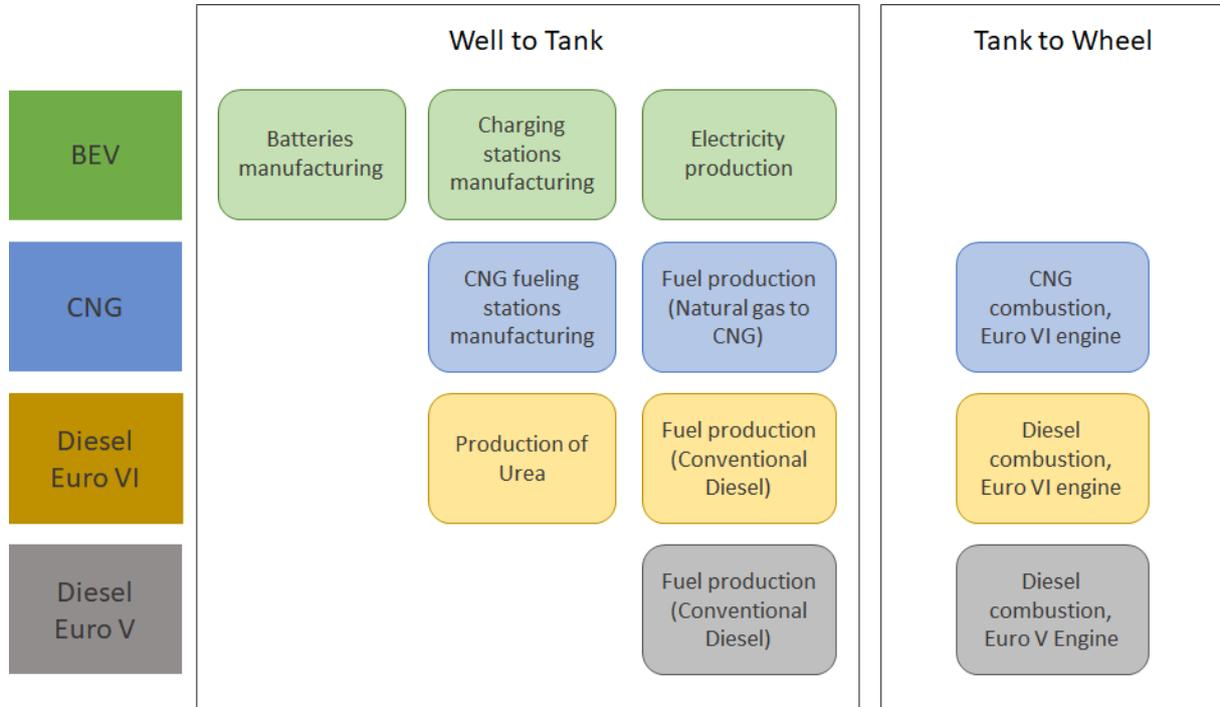
Figure 1. Activities included in calculation of WTT (CO<sub>2</sub>eq) and TTW (CO<sub>2</sub>eq, NO<sub>x</sub>, PM<sub>10</sub>) emissions
