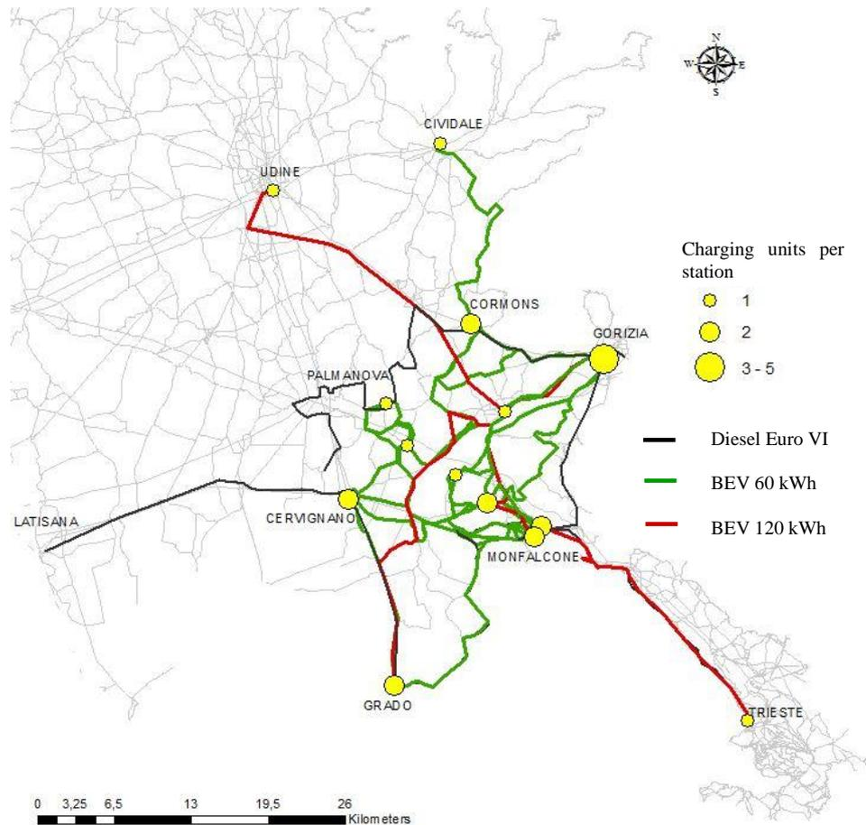
Figure 4. Map of optimal system configuration for - 50% CO<sub>2</sub>eq scenario.
