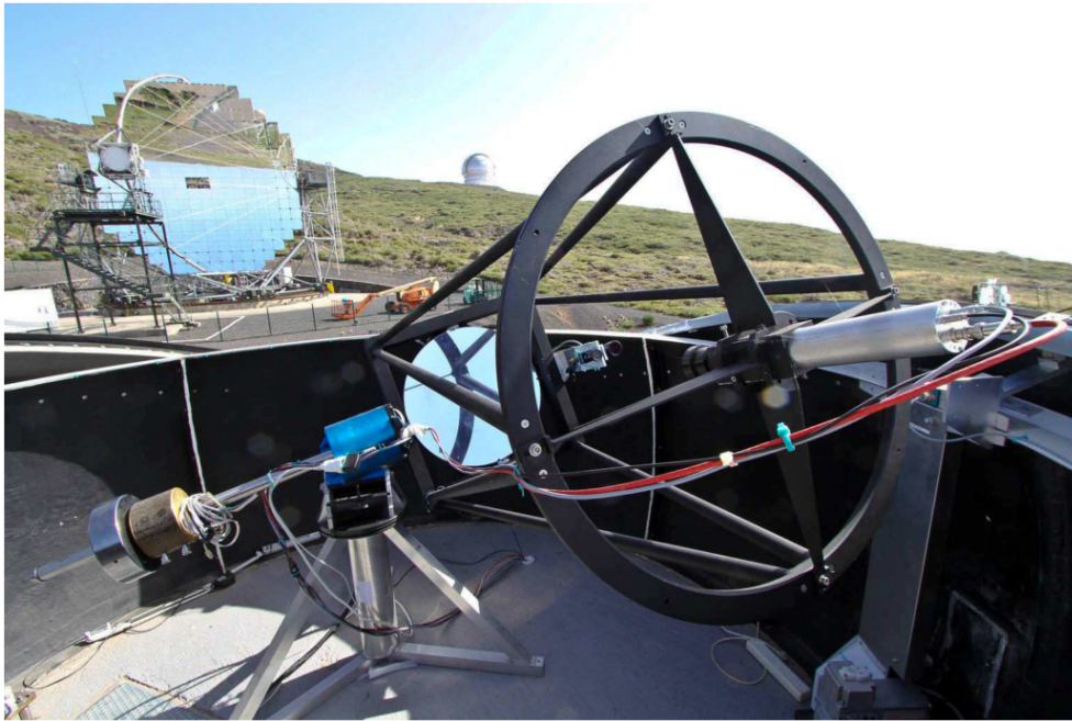
Figure 8: The MAGIC ‘micro’ LIDAR system in its dedicated dome on top of the MAGIC counting house [48].
