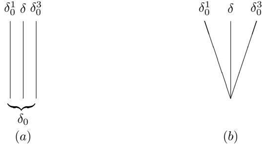
Figure 4: A composite wave \delta_0 in the (x, t) -plane: in (a) it is drawn as three parallel close lines, while the auxiliary picture (b) is used to determine the states in the interactions.
