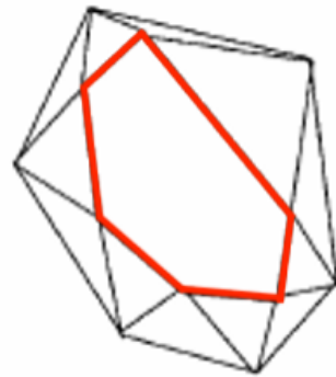
(a) Holes (Missing triangles).
