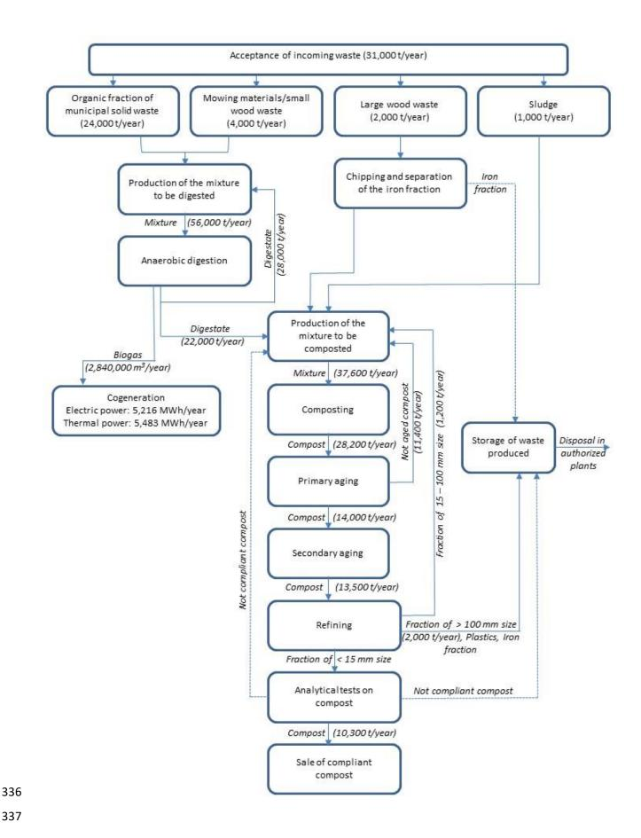
Fig. 1. Matter balance foreseen for Degas Ecologia plant
