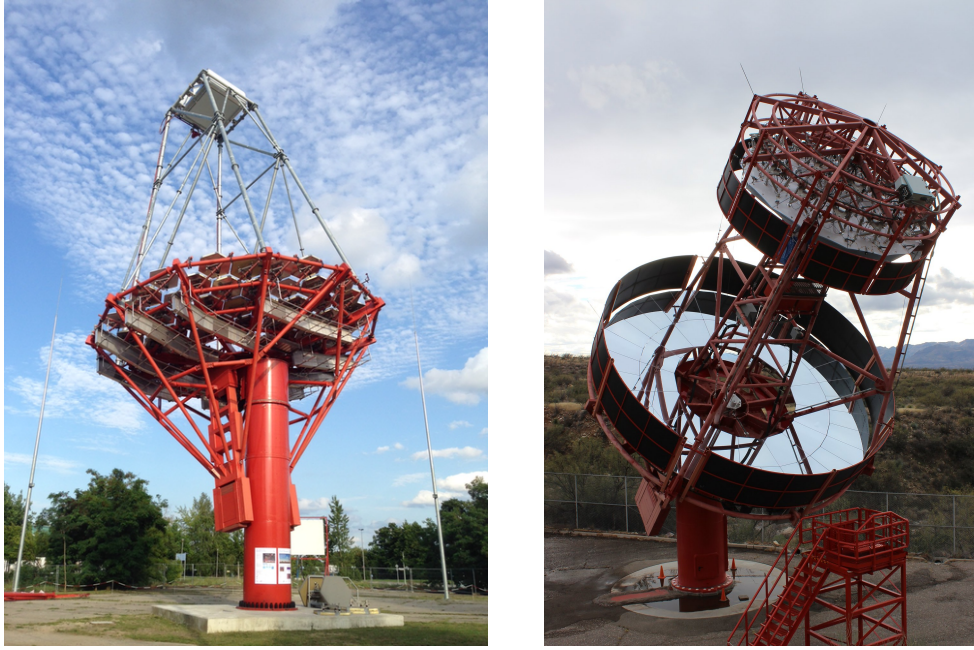
Figure 3.4: DC-MST prototype equipped with FlashCam in Berlin-Adlershof (left) and SC-MST prototype at the Whipple Observatory in Arizona (right). Figures from https://www.cta-observatory.org
