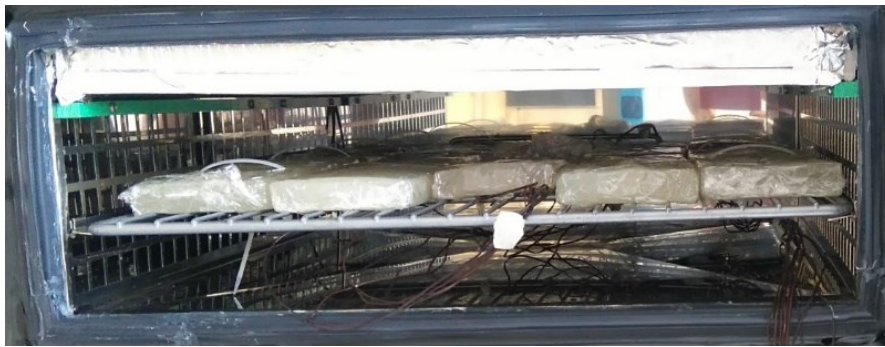
Fig. 17 Schematic representation of chicken fingers bag and Tylose bricks on grid (top) and grid loaded in air impingement prototype thawing chamber (bottom).
