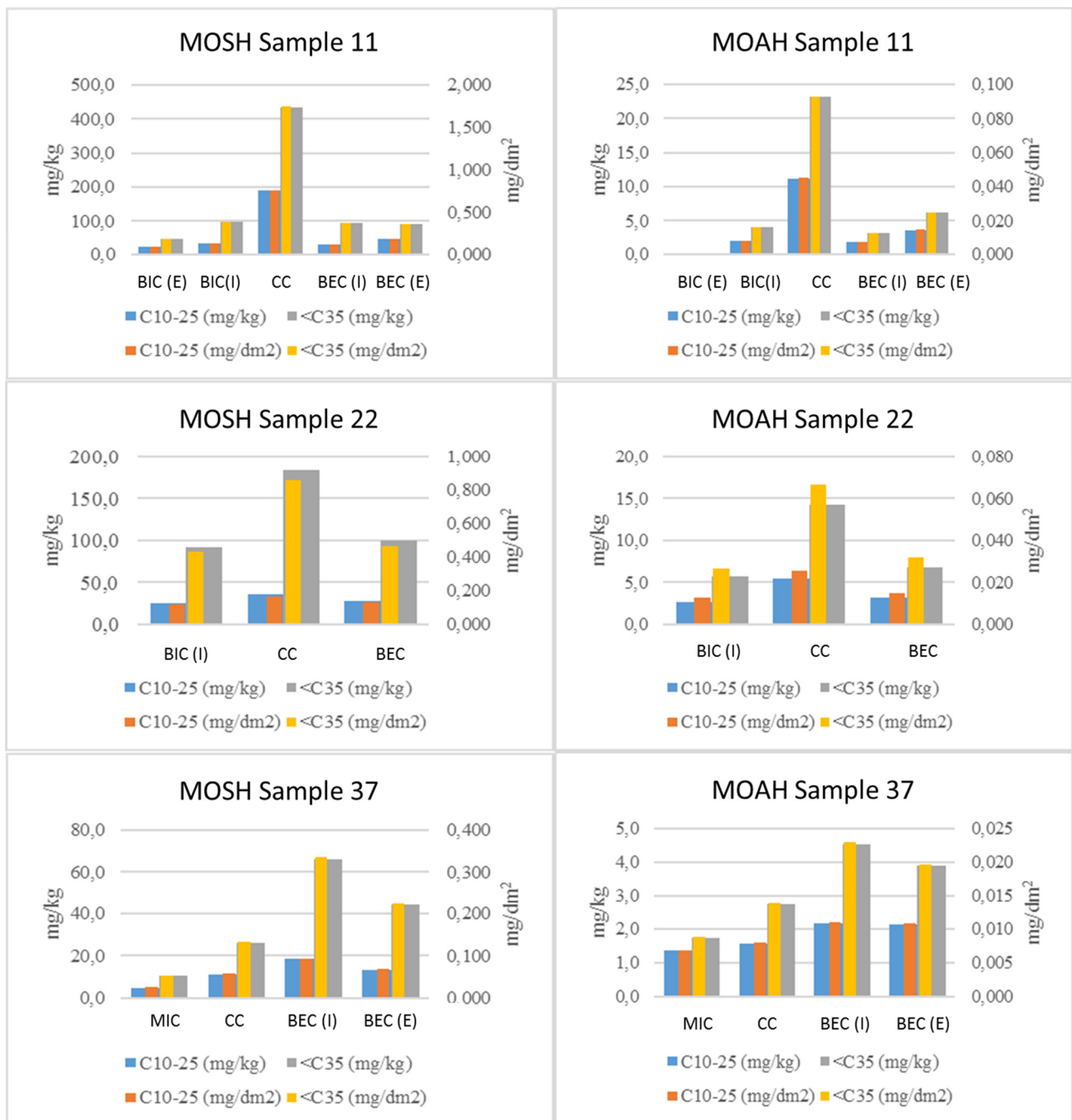
Figure 25. Concentration of MOHs (C 10 -C 25 and <C 35 ) in different layers of sample 11, 22, 37.
