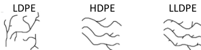
Figure 2. Microstructure of low density polyethylene (LDPE), high density polyethylene (HDPE) and linear low-density polyethylene (adapted from ref:[11]).
