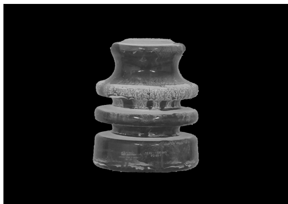
Figure 2. Conversion of the photograph of the insulator sample after segmentation.
