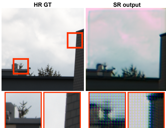
Figure 5.7: Imprecise warp matrix. All images are converted from raw sensor space to sRGB for visualization purpose.
