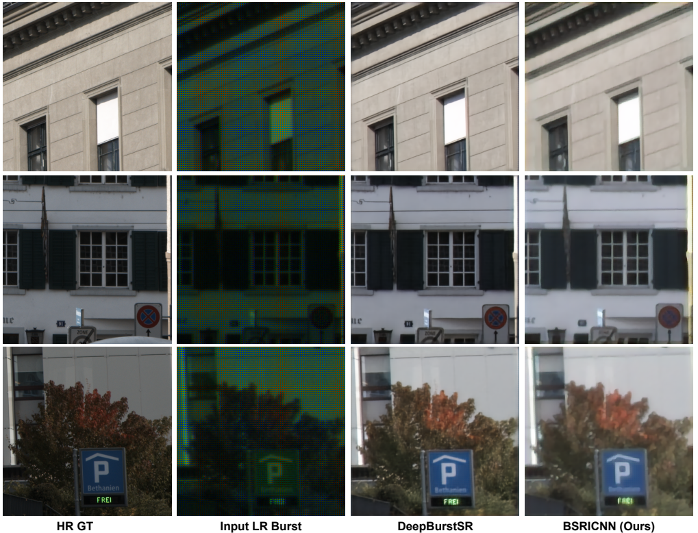
Figure 5.6: SR visual comparison of the proposed BSRICNN method with the existing Burst SR methods on the real-world BurstSR testset at the \times 4 upscaling factor. All images are converted from the raw sensor space to sRGB for visualization purpose.
