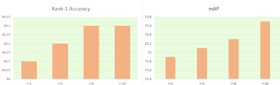
Figure 3.15: The impact of choosing different values for the reduction ratio r on DukeMTMC-reID dataset. Left side represents the rank-1 accuracy scores and right side shows the mean average precision (mAP)
