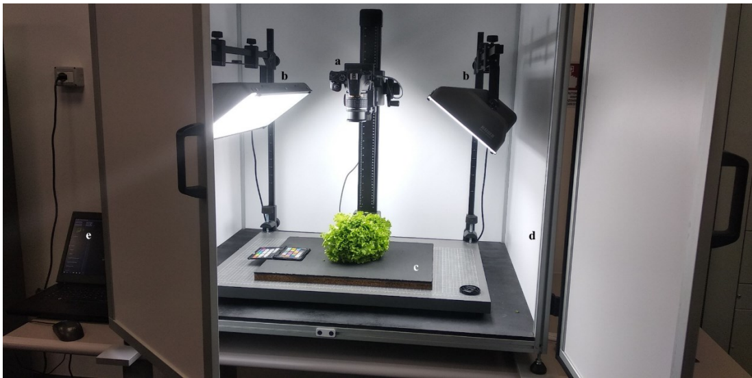
Figure 20 Color imaging system: (a) color digital camera, (b) lighting system, (c) matte black soft pad, (d) photo chamber, (e) computer directly connected to the digital camera.
