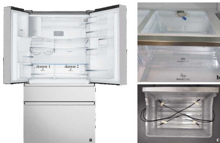
Figure 13 Refrigerator model (a), position of the ionizer in drawer 2 (b), and probes position for the monitoring of temperature and relative humidity (c).
