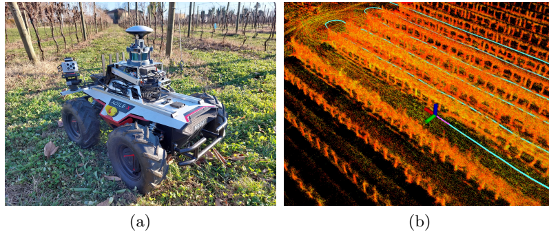
Fig. 3: Scout 2.0 mobile robot (a); 3D reconstruction of the vineyard (b).
