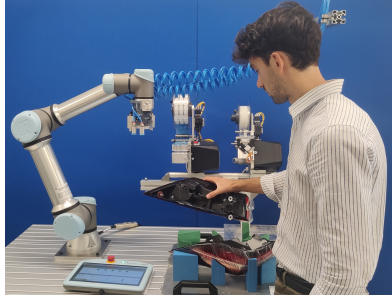
Fig. 4: Example of human-robot collaboration for an assembly task.
