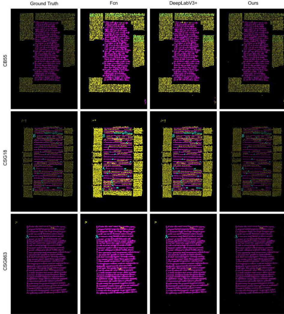
Fig. 6: Image showing a qualitative comparison between our framework and the competition ones. Each row represents a zoomed area belonging to a different instance of the dataset, representing the three classes of manuscript contained in it. In the first column, the ground truth segmentation maps for the 3 images are shown, while on the remaining columns we provide the results produced by the three systems, FCN, DeepLabV3+ and Ours respectively
