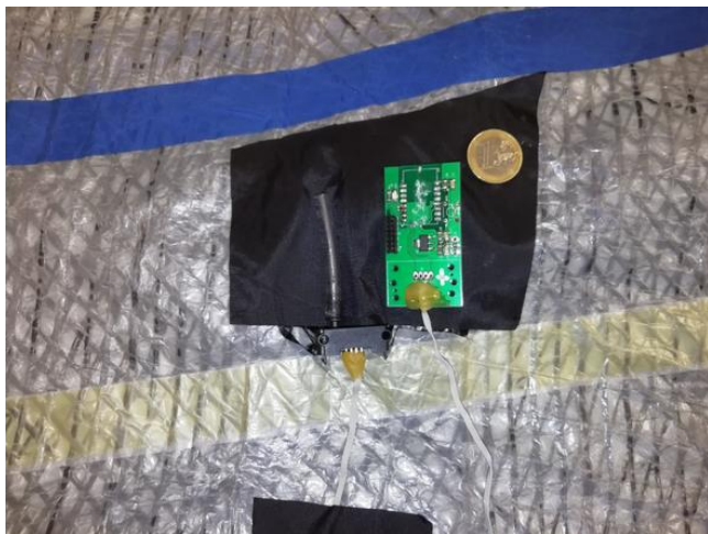
Figure 3. PCB realization of the wireless pressure sensor mounted on the sail.
