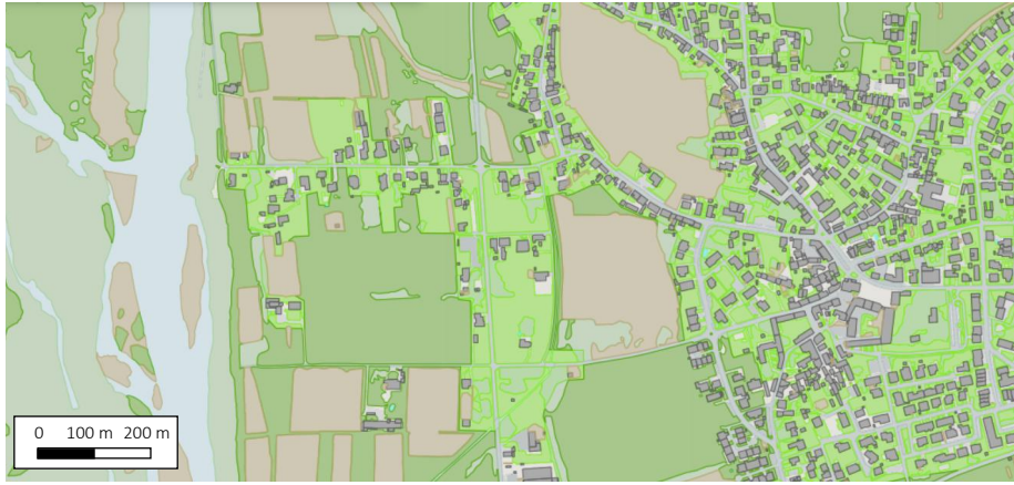
Fig. 6: Simplified version of the DBT (DBTsped), obtained directly from the true orthophoto. Only the most interesting classes are retrieved.
