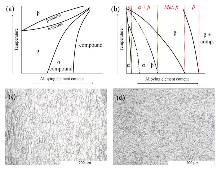
on beta transus temperature. The role of alpha and beta stabilizers in the control of the microstructure of titanium alloys is summarized in Figure 2.
