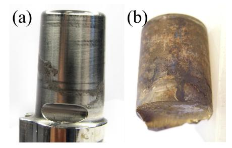
**Figure 7.** Examples of (**a**) fretting damage after 5 years in vivo and (**b**) mechanical failure due to fretting corrosion after just 2 years in vivo for Ti-6Al-4V tapers in modular femoral stems.
