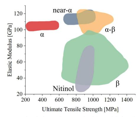
**Figure 3.** Relationship between ultimate strength and elastic modulus for a selection of alloys commonly applied in the biomedical field, grouped by chemical composition.
