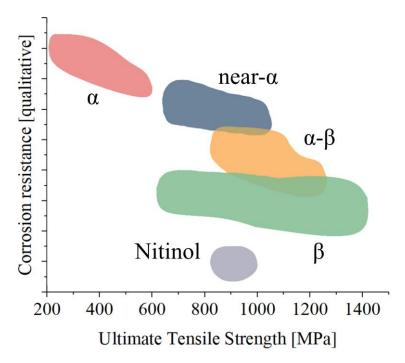
**Figure 4.** Relationship between the ultimate tensile strength and the qualitative corrosion resistance of titanium alloys applied in the biomedical field. The colored areas indicate the kind of alloys.
