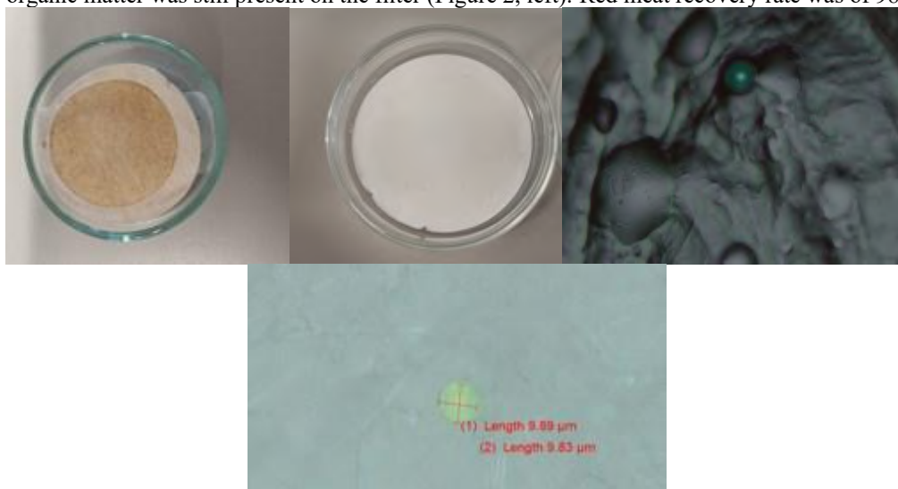
Figure 2 Filters after digestion and filtration of pasta, using Fenton's Reagent (left) and meat sample, using KOH 5M (centre) and polystyrene fluorescent microbead before (on meat sample) and after digestion and filtration (right).
